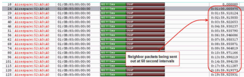
Figure 2: Neighbor Messages are sent every 60 seconds to the multicast address of 01:0B:85:00:00:00.
